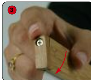
Rotate the end cap closed
